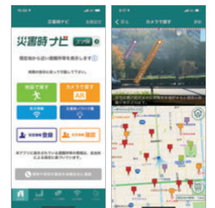
SmaHo Emergency Navigation uses GPS and an AR camera. On the street view, an arrow indicating the route enables tourists unfamiliar with the area to find their way to the nearest shelter.
