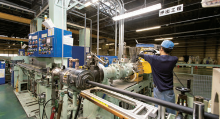
In this process, melted rubber is pressed around the steel mandrel to build the base layer of the hose.
